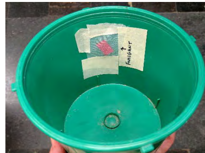
Hercon vaportape HC-8500-25 note: vaportape has an embedded fumigant
